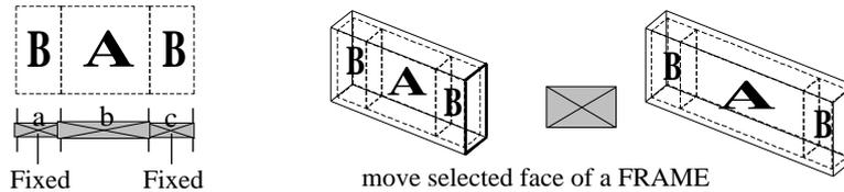
Figure 14. Scaling a FRAME in condition that size of sub-FRAMES are fixed
