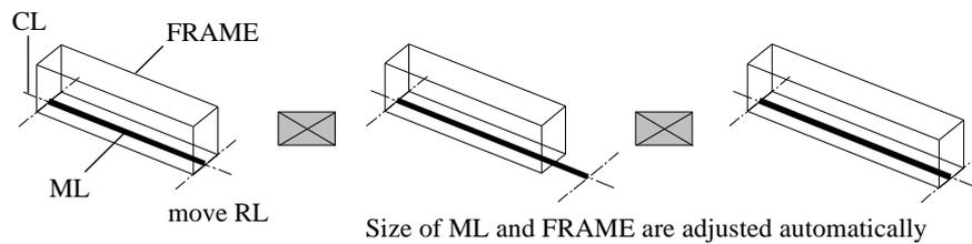
Figure 7. Image of Adjusting a ML and a FRAME by moving Construction Line
