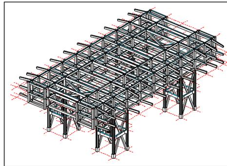
5) Members of the core are exposed by glass. Study custom shapes of the members of the core from architectural and structural factors.
