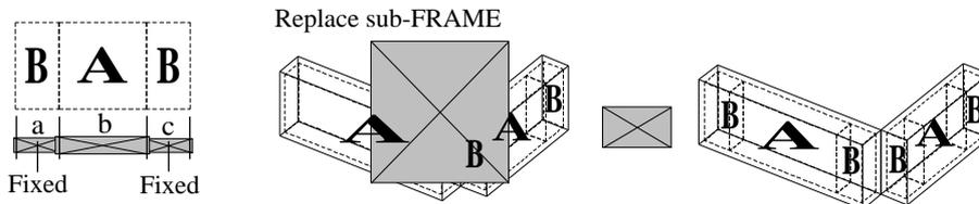
Figure 13. Replacing sub-FRAMES in condition that size of sub-FRAMES are fixed
