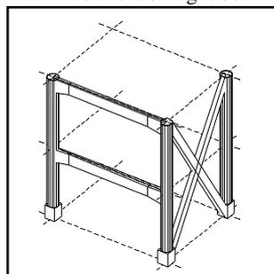
9) After attaching the data to the sub-FRAMES that represent the haunches so that the length of haunch is set, the translation of CLs causes the size of the beams to increase while the length of haunches does not change. (CLMV)
