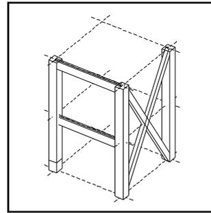
3) After defining a sub-FRAME in a FRAME (MKSUBFRM), divide it into two sub-FRAMES.(DIVSUBFRM)
