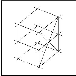
1) Draw CLs and MLs by considering the structural conditions. (CLINE, MLINE) Each ML represents the location of columns, beams, or braces.
