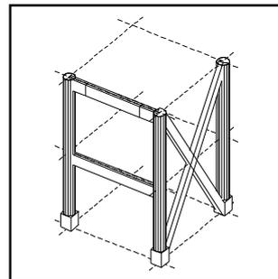
6) Define a sub-FRAME in each of the horizontal FRAMES, then divide the sub-FRAME of the upper beams into 3 sub-FRAMES that represent haunches and a straight beam.
