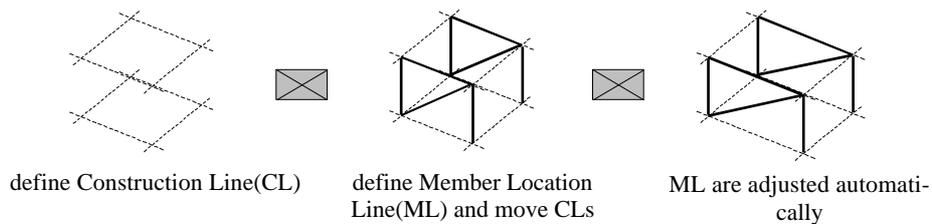
Figure 5. Image of Adjusting Member Location Lines by moving Construction Lines
