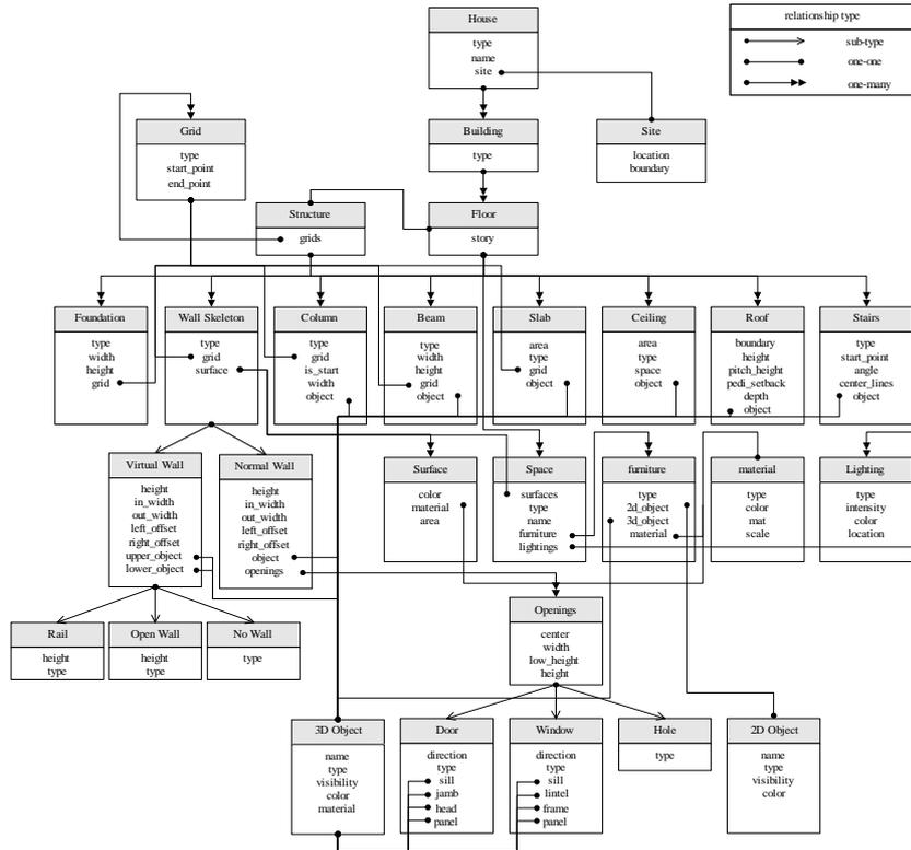
Figure 8. A Building data model (Choi, 1997, Quote from Hwang, J-E. 2002, SpaceScope: Developing a Spatial Information Retrieval System -Focused on Apartment Unit Floor Plans)
