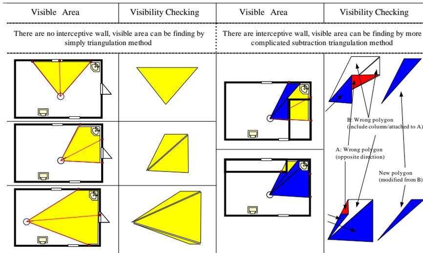
Figure 4.3. The process of visibility checking
