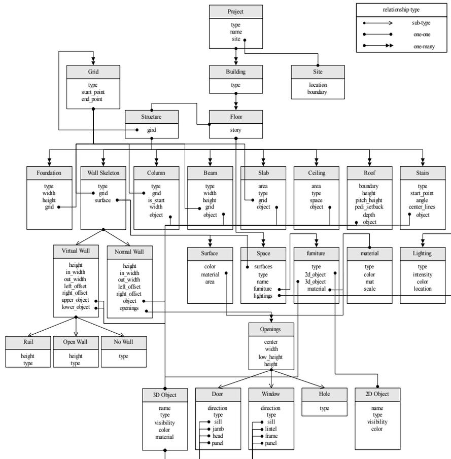
Figure 4. The building data model for the object-oriented CAAD system
