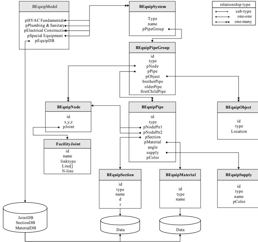
Figure 7. A data model for building equipment
