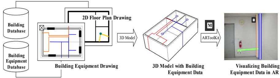
Figure 8. Process of building equipment visualization
