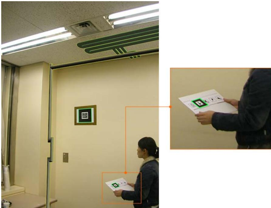
*Figure 10. AR experiment using artistic frame marker and slider marker*
