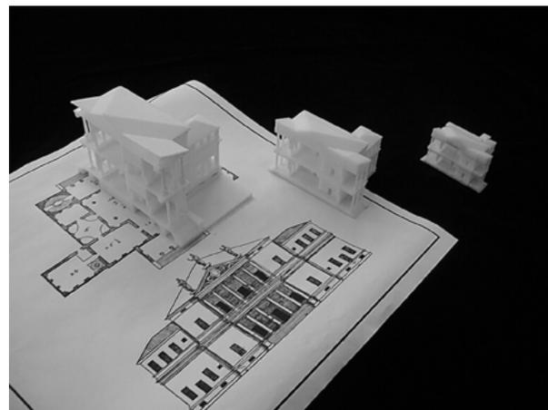
Figure 11. 3D printing techniques used to view models in physical form. Smallest model is a sketch representation with very little detail; largest model is a detailed representation of the villa showing column and ornamental details
