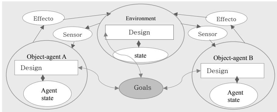
Figure 3. A conceptual structure of a self-organizing design environment
