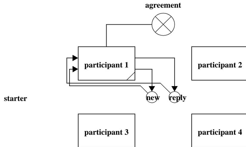
When the agreement is set the project can start. All participants are connected by four channels: one channel of type “new” and one channel of type “reply” on the input side and on the output side. The “starter” of the process sends a message of type “new” that contains the start state of the building product and the desired end state of the building product.
