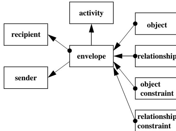
The functional data model of Figure 31 shows the envelope with its attributes and the contents of the envelope, the product model. The product model is represented by the basic concepts of object-oriented modeling, namely objects, relationships (between objects) and constraints (on objects and relationships). “Reply” messages do not contain the sender entity and the activity entity.
