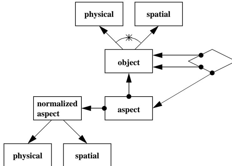
Using functional data modelling in Figure 28, the object decomposition relationship is presented by an association entity. The association entity references an aspect from the normalized set of aspect types. Whereas an object is either “physical” or “spatial”, aspects can often be used in both circumstances but not always. A relationship always references an aspect that is common to the two related objects.
