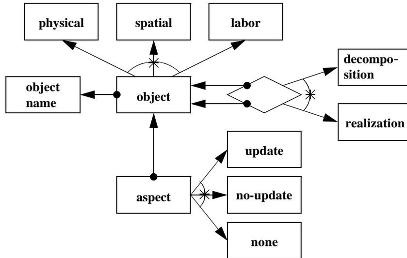
Since process description can evidently not be represented by functional data modelling, the third task description method is not presented in Figure 30. The association entity that relates two objects now can be of type “decomposition” or “realization”. Every aspect of each object in a “task” or “request” description will have one of the three operation attributes.
