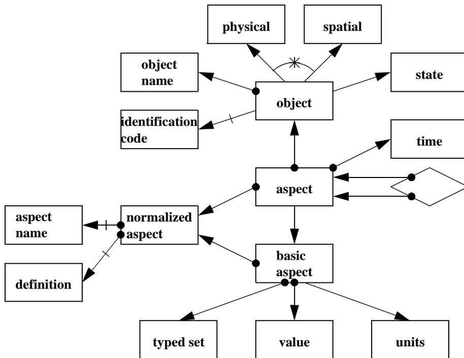
Most considerations about objects and aspects are presented in the functional data model of Figure 27. Central part is of course the object with one or more aspects associated to it. Note that the object can have any object name, whereas the aspect must be chosen from an aspect type set. Aspects are decomposed using the association entity. Every aspect has a time stamp indicating its creation or updating time.
