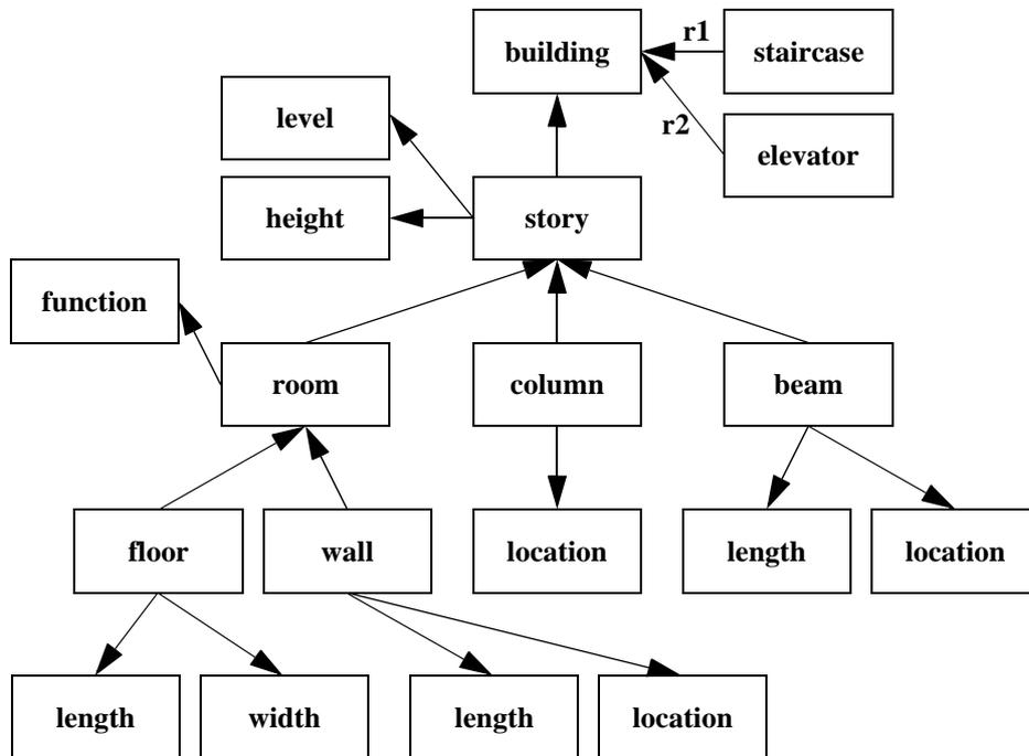
The source data structure of Figure 19 describes a preliminary design of a small office building. A simple line drawing of each story is available including the ground floor. The primary focus of this representation is the area of rooms, their dwelling function and their location.
