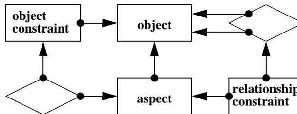
In the functional data model of Figure 29, an object constraint is associated to one or more aspects of a certain object. Each relationship constraint references an object decomposition relationship and a specific aspect. The relationship constraint in fact replaces the direct reference from the object decomposition to an aspect (see Figure 28).
