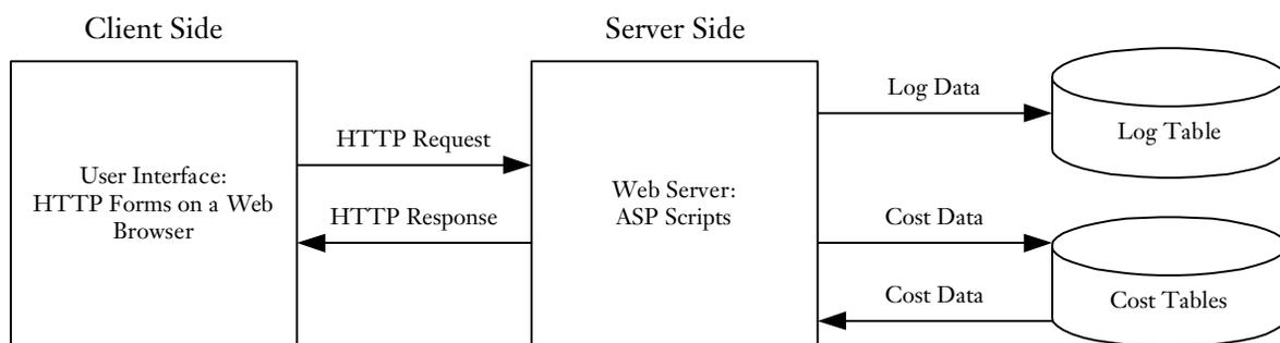
Figure 1. Software components of the Web-based cost estimating tool.
