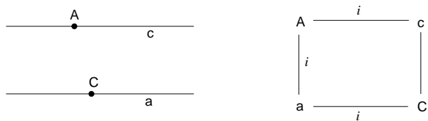
Figure 3.5 Incidence of A with a and C with c and resulting constraint graph.
