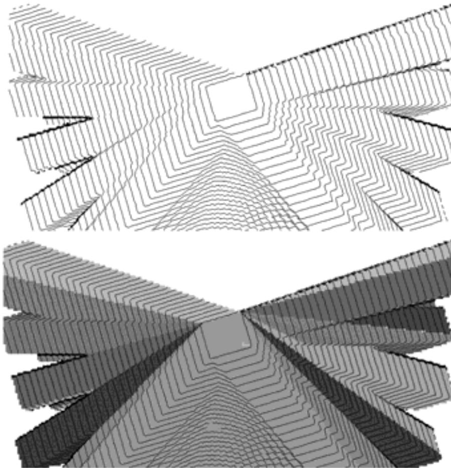
Figure 3. Representations of solar fan as a contour map (top) and as a contour map related to influencing months (bottom). This figure illustrates the wave effect due to sampling period.
