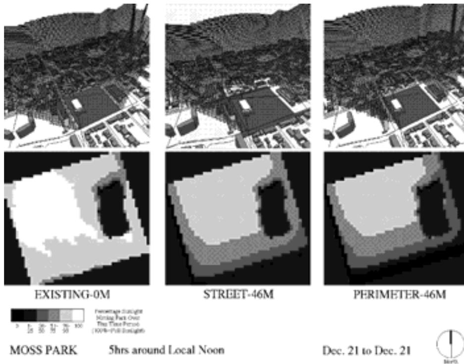
Figure 7. Solar Fans And Associated Solar Raster Maps For A Typical Study Site.
