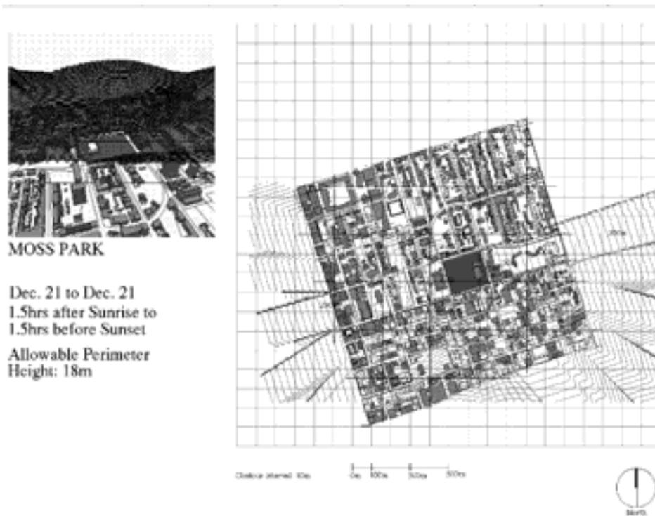
Figure 6. Solar Fan And Contour Map For A Typical Study Site.
