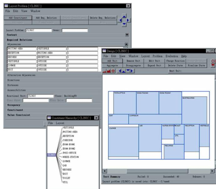
Figure 1. A snapshot of the SEED-Layout environment.
