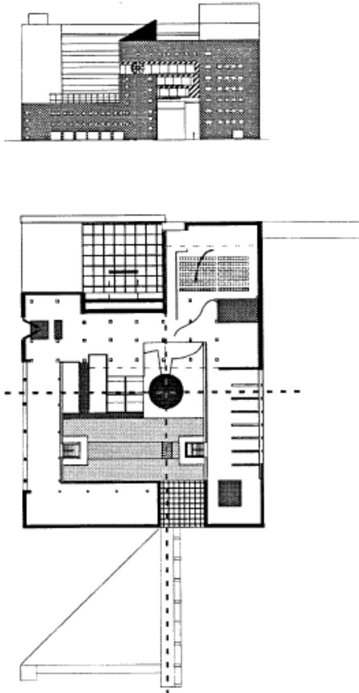
**Figure 7.** Ground floor plan and front elevation at an early stage of the design process.
