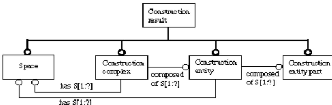
FIG. 8: Relations of the concept of space to other construction results according to ISO
