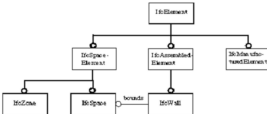
FIG. 10: An IfcSpace is seen as bounded by an IfcWall
