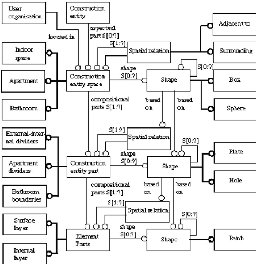
FIG. 14: Principle structure of a comprehensive schema of construction entity space
