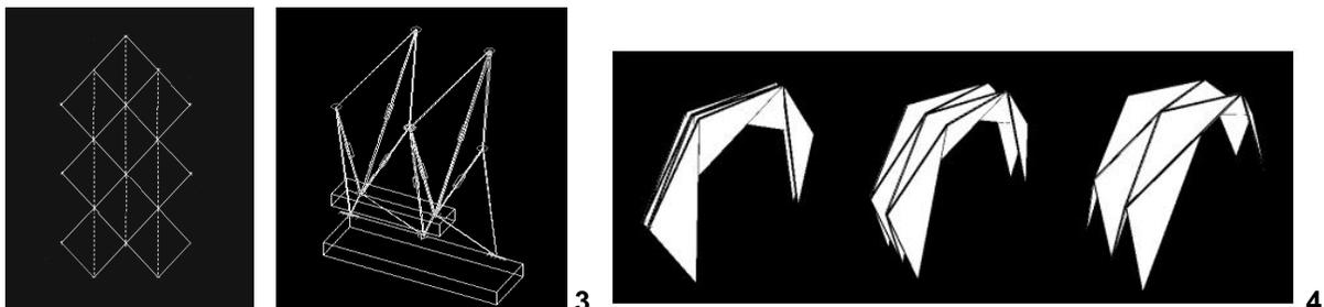
**Figure 3:** Kinematic analysis simulations of a 16 tile structure
