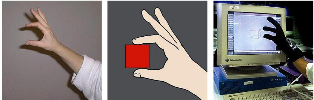
Figure 5. The hand formation is recognized by the system and a solid is associated to it, as if the user were holding the object. Once virtually grabbed, this object can be positioned with one hand movement, or scaled just with the aperture of the fingers, i.e., if the fingers are brought closer to each other, the model is scaled down, if the hand is opened, the model is enlarged.
