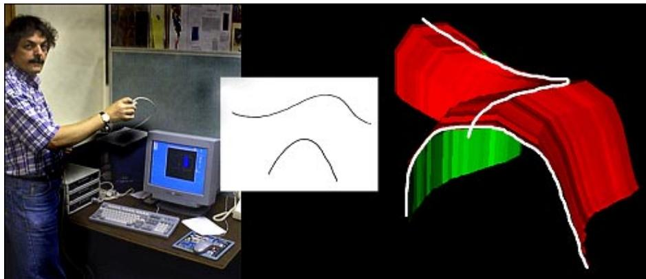
Figure 2. The tracker has a sensor (inside a mouse box) which receives the magnetic emission of another box, the tracker's coordinate origin. The sensor's spatial position is sent to the controller in 144 Hz, i.e. 144 times per second. This position information is then transformed by the software in graphic form. In this case, the software draws lines with the movements of the receiver.
