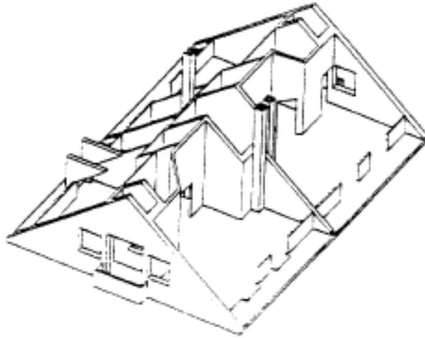
Pict. 3. Axonometric view of roof -level without roof-cover:
