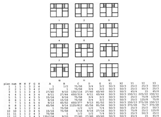
Figure 5. Schematic Plans for the Villa Angarano Typology ( $P = 3/4$ , width = 50 feet, stair width = 7 feet)
