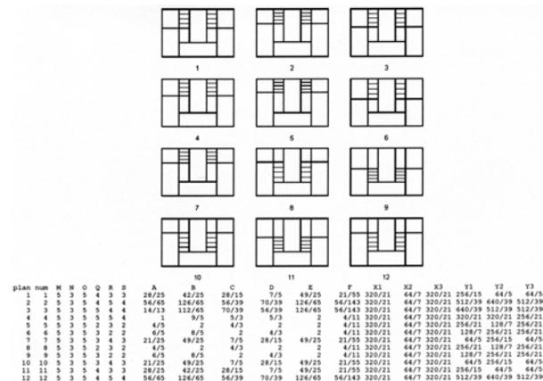
Figure 7. Schematic Plans for the Villa Badoer Typology (P = 2/3, width = 64 feet, stair width = 7)
