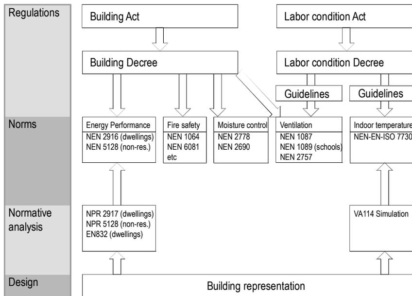
Figure 1. Requirements complexity: Dutch norms and regulations on indoor climate
