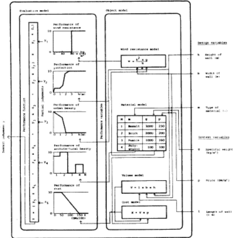
Fig. 4. Planning model for a wall serving as a fence
