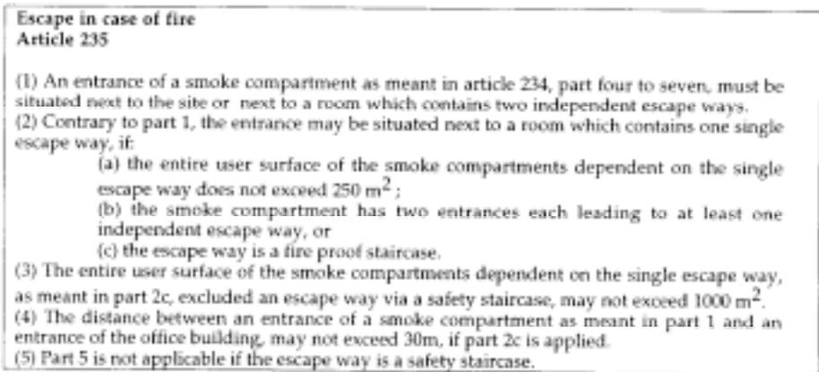
Figure 4: A part of Article 235 of the Dutch Building Regulations
