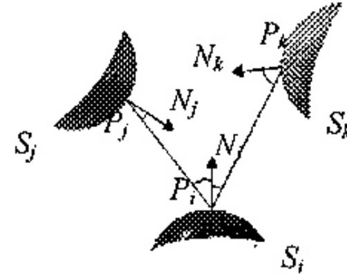
Radiosity (Goral et al. 1984), thermodynamics offers the physical background to this algorithm: every surface is considered as part of a Lambertian body, which reflects light with equal intensity in all directions. The algorithm subdivides each polygon into ever smaller unitary elements and computes for each of them the sum of the energies emitted by all the others. The resulting equation system (3) represents the interchange of energy of the environment, both reflected and emitted.
