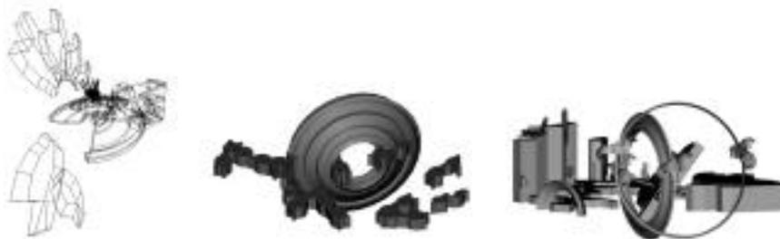
Figure 7. Creating a ‘spatial entity’ by applying Boolean operations to selected 3D objects.
