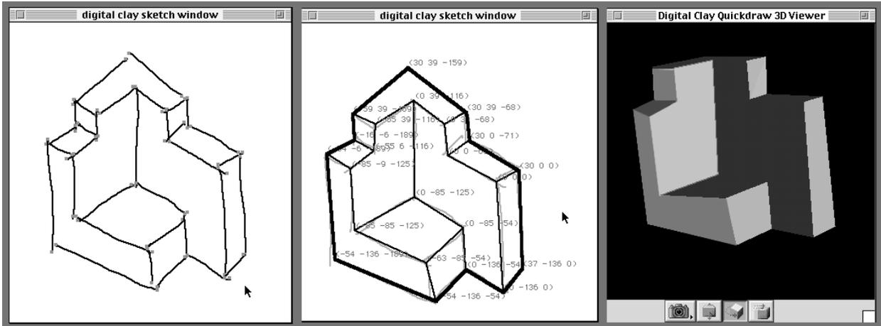
3. Digital Clay converts freehand sketches into 3D model (E. Schweikardt)
