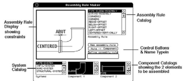
1. Interface for making assembly rules in Construction Kit Builder (M. D. Gross)
