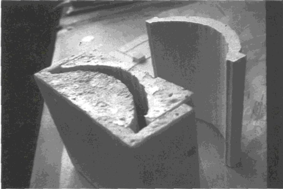
The one-cut exercise. After the foam block is cut once with a hot wire cutter, the two pieces are displayed to create a formwork void for casting the prototype element in plaster.
