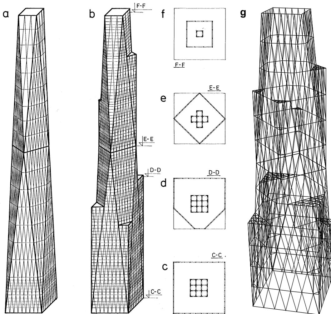
Figure 3. General schemes of exemplary forms of tall buildings designed by means of structural system called framed polyhedron
