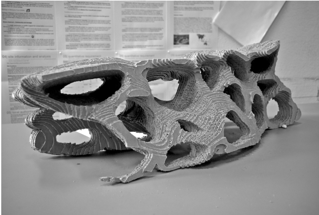
Figure 3. Cardboard CNC fabricated prototype of student work in the Digital Design Studio (Author)
