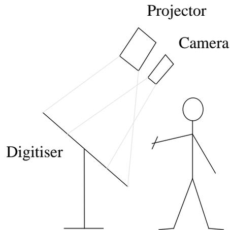
Figure 2. The Digital Drawing Board
