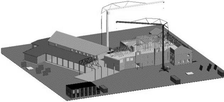
Figure 1: Visual simulation of construction process. Support for site and work planning.
