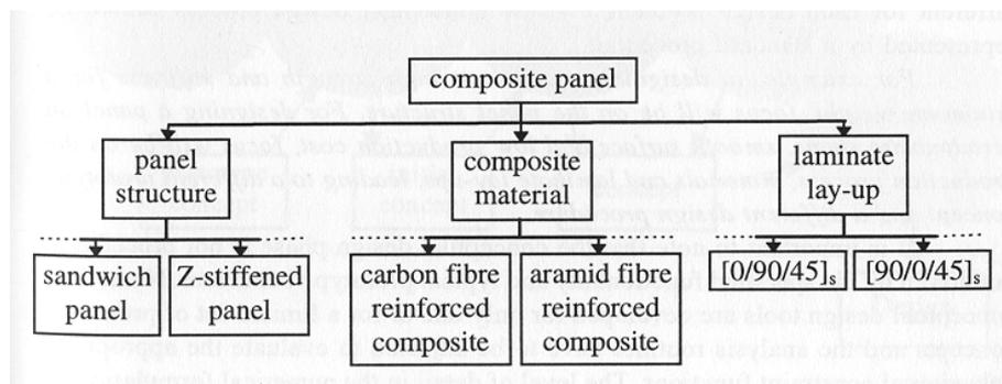
Figure 1: Breakdown of a panel prototype in design elements
