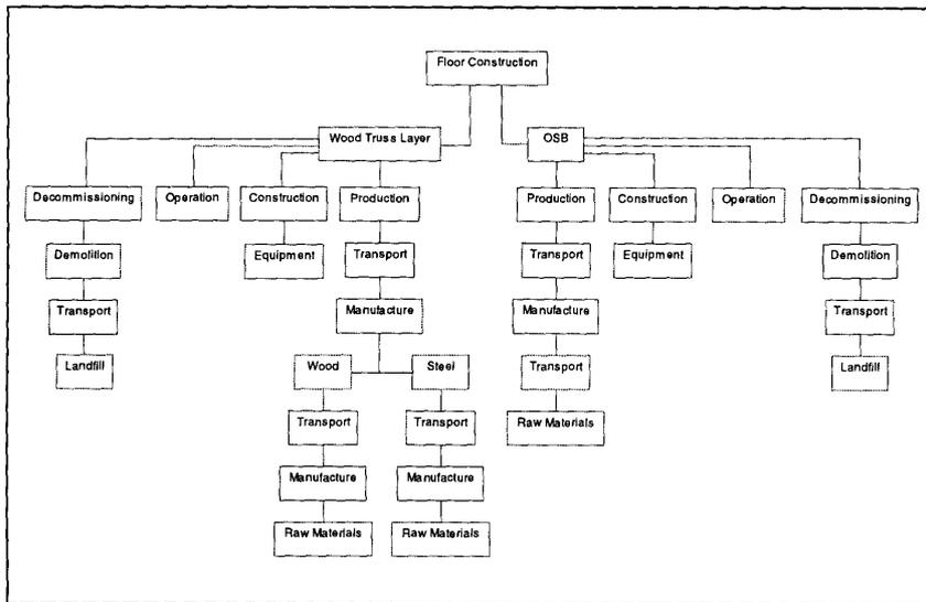
Figure 3. Partial representation of a floor construction in ECOLOGUE
