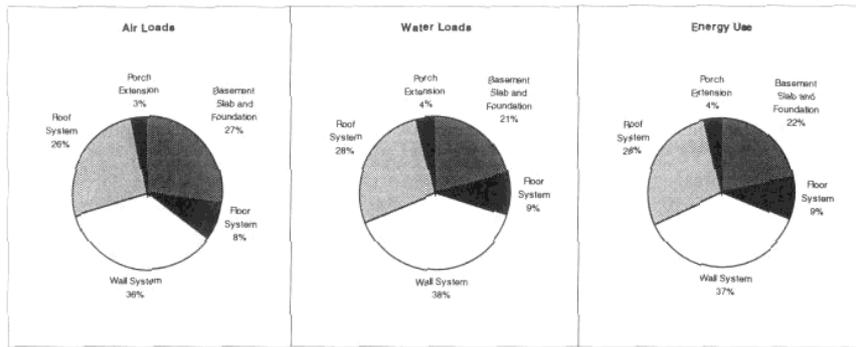
Figure 5. Distribution of loads for the construction phase
