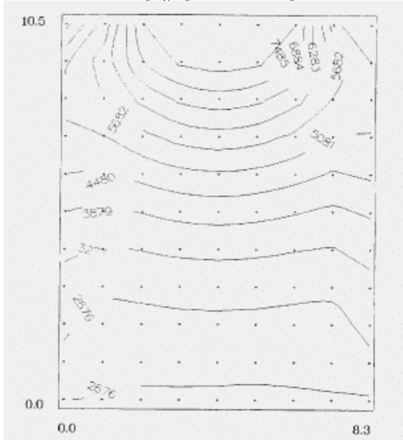
Fig. 5 Daylight factor contours for Illuminance on the East wall of Studio 38.
