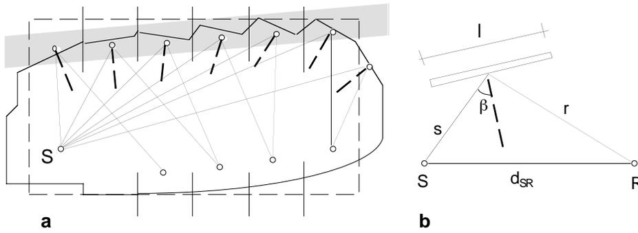
Figure 1. Illustration of a rule-based approach to acoustical design of concert halls (a) and schematic illustration of the determination of reflector sizes (b).
