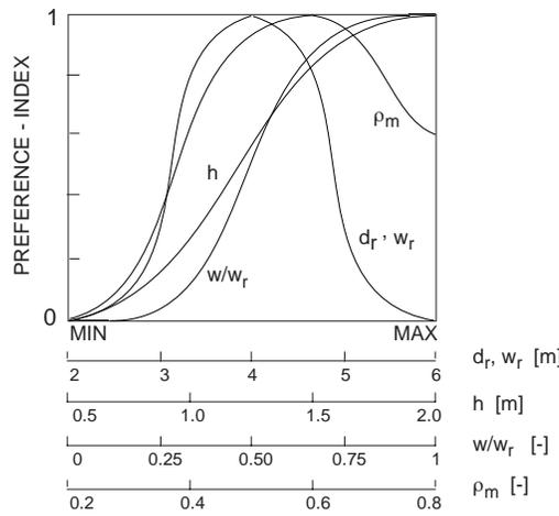
Figure 7. Preference-indices for five daylighting design-related variables implemented in GESTALT. ( $d_r, w_r$ : room depth and width,  $h$ : window height,  $w/w_r$ : window width to room width ratio,  $\rho_m$ : room average reflectance).
