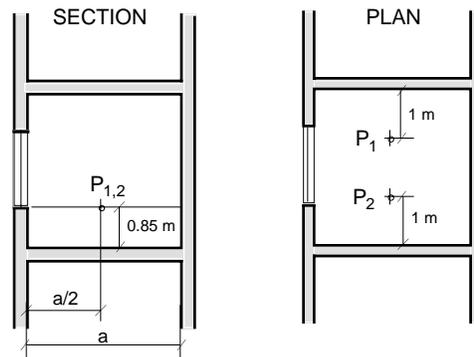
Figure 6. Reference points for the evaluation of daylighting (after DIN 5034).
