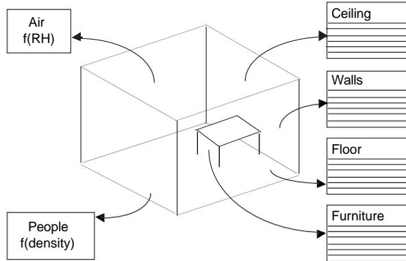
Figure 2. Schematic illustration of data base components pertinent to the design and evaluation of the reverberant field in a room.
