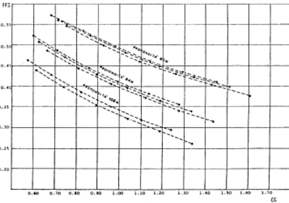
FIG.9. Graphs solar heating fraction (FFI, FFD) Trombe wall type, position 1.
