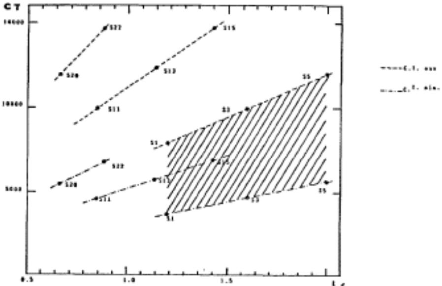
FIG.7. Graphic CT-L/P.Type position 1. The dotted lines shows the variation area of thermal load among houses with steady depth. CTthermal load; L,P= leught and dept.
