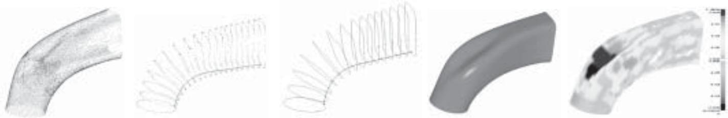
are then used to generate lofted NURBS surfaces (figure 3.4d). The resulting surfaces can be compared to the scanned point cloud for an analysis of deviations from the original physical model (figure 3.4e).
