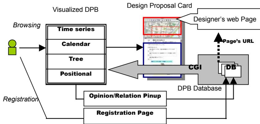
Figure 3. Structure of Design Pinup Board
