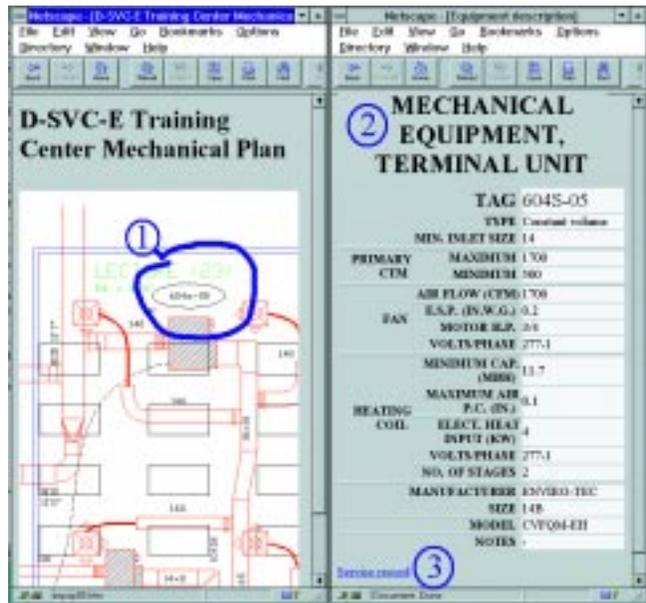
Figure 3. Retrieving operations information using Web technology.
