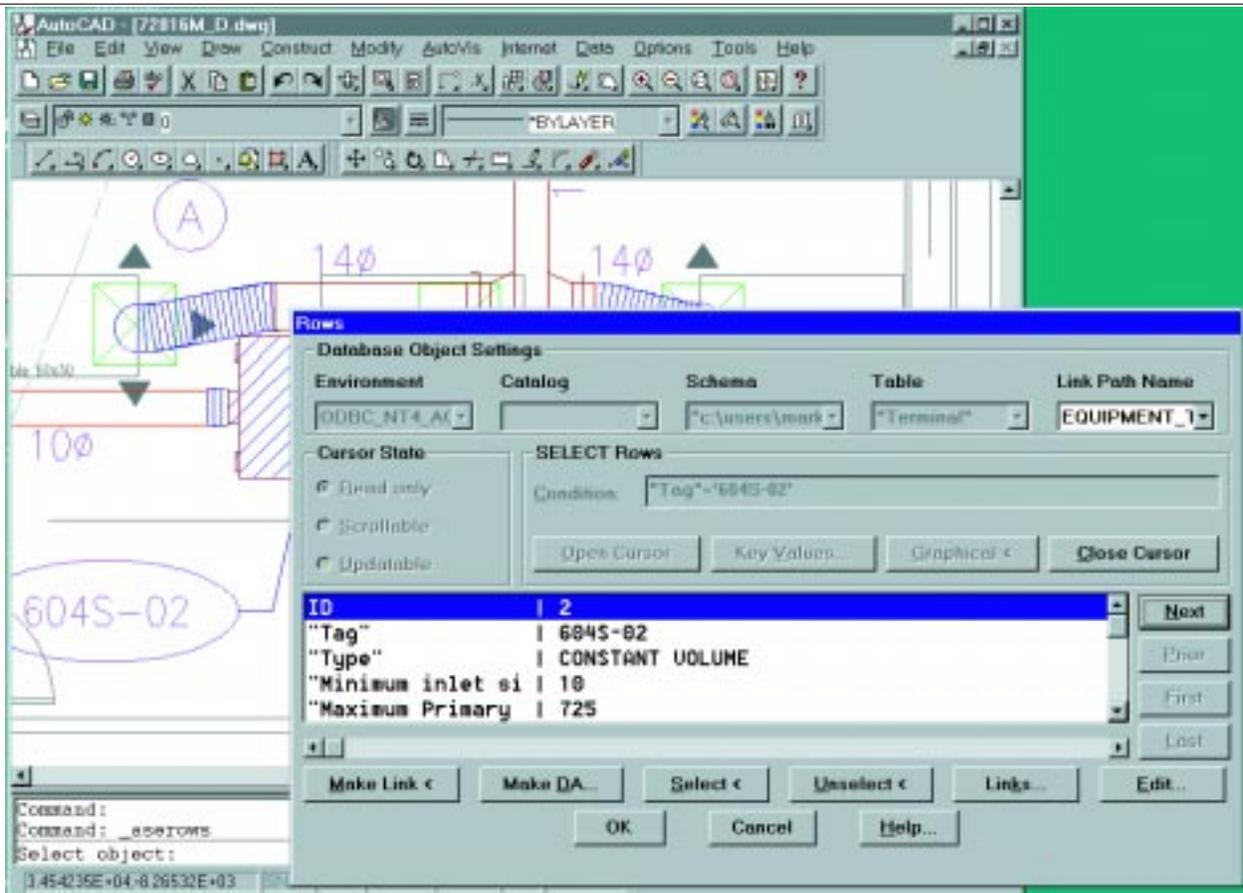
Figure 4. Retrieving operations information from within CAD software.
