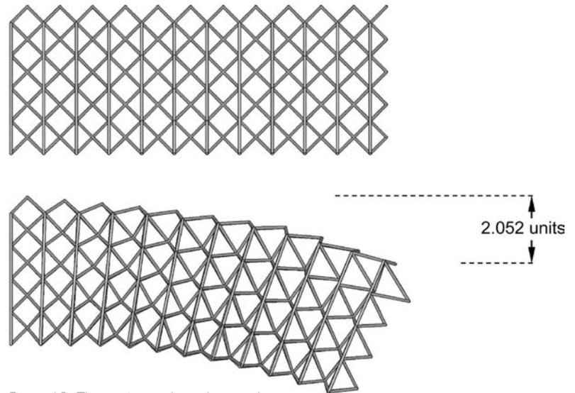
Figure 12. The engineered topology, and the resulting deformation under loading
