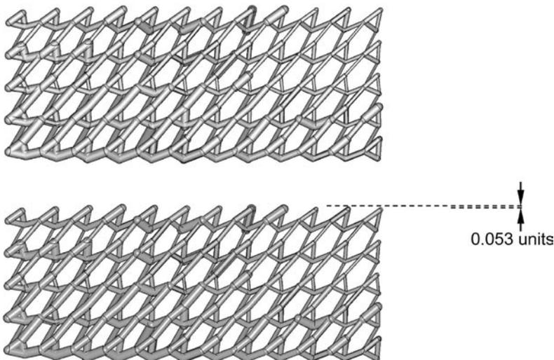
Figure 15. The evolved topology, and the resulting deformation.
