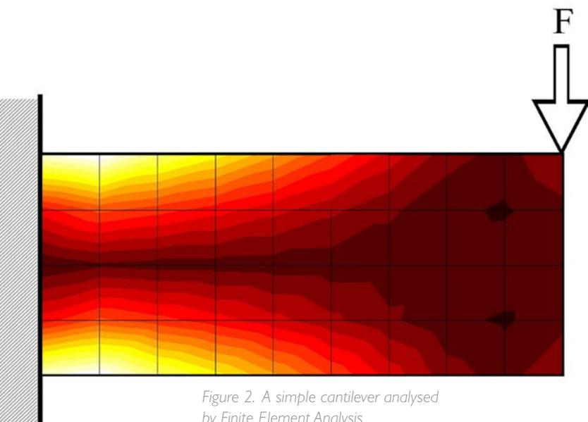
Figure 2. A simple cantilever analysed by Finite Element Analysis
