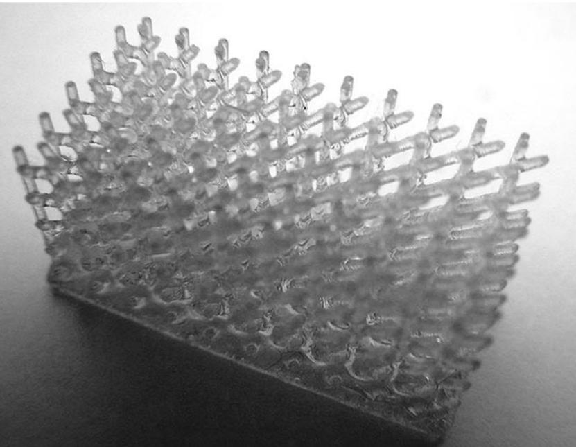
Figure 3. A sample microstructure fabricated by stereolithography
