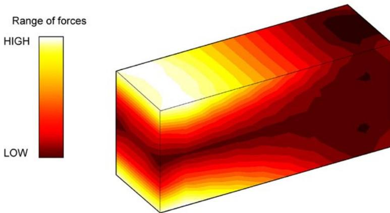
Figure 6. The cantilever as analysed by Finite Element Analysis
