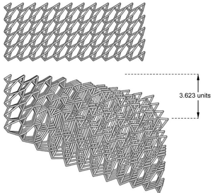
Figure 13. The evolved topology, and the resulting deformation under loading
