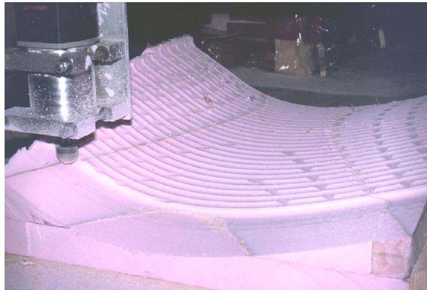
Figure 6. CNC-milling of a foam mold
