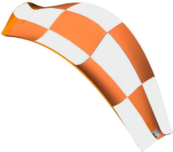
Figure 2. Subdividing a parametric shell model into segments
