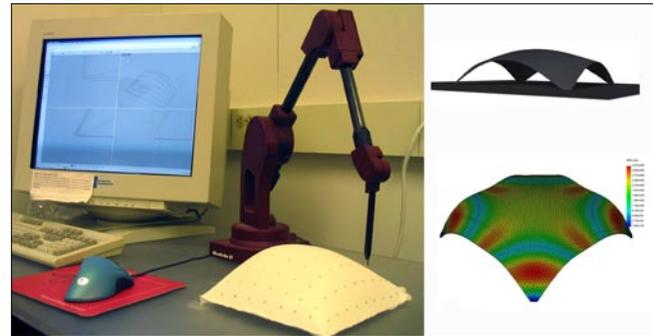
Figure 3. Left: Digitizing a conceptual physical shell model. Laser scanning techniques (not shown) are commonly used for final, accurate measurements. Right: results of computational form-finding techniques using the general finite-element method.
