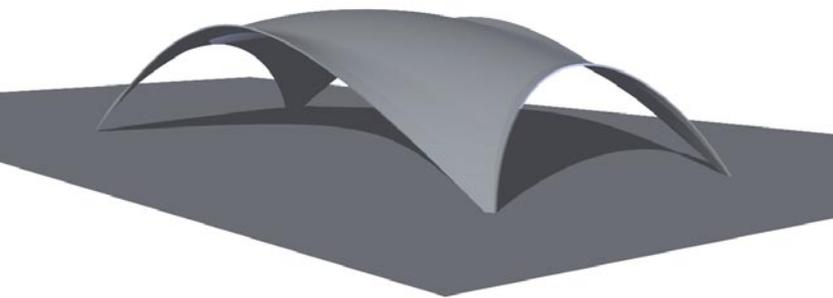
Figure 11. Parametric model of Isler's shell
