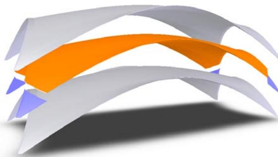
Figure 12. The components of the concrete sandwich shell in exploded view
