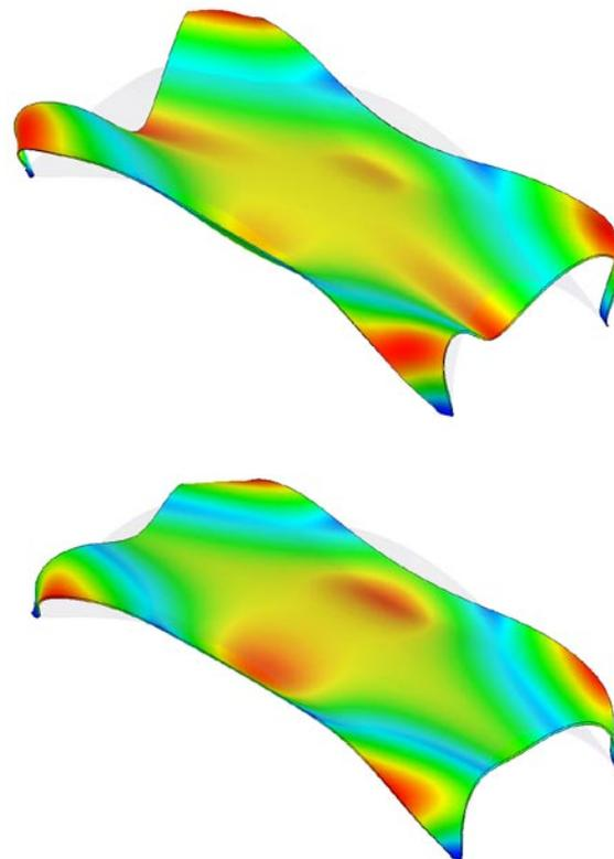
Figure 4. Comparative FEA deflection study of a shell: Model 1 on the left has increased thickness near the supports; Model 2 on the right has constant thickness. The deflections are shown magnified by a factor of 50. Model 2 has much larger deflections, especially near the supports.
