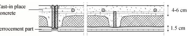
Figure 10. Cross-section through a Ferrocement-Concrete Sandwich shell: a segment joint shown on the left
