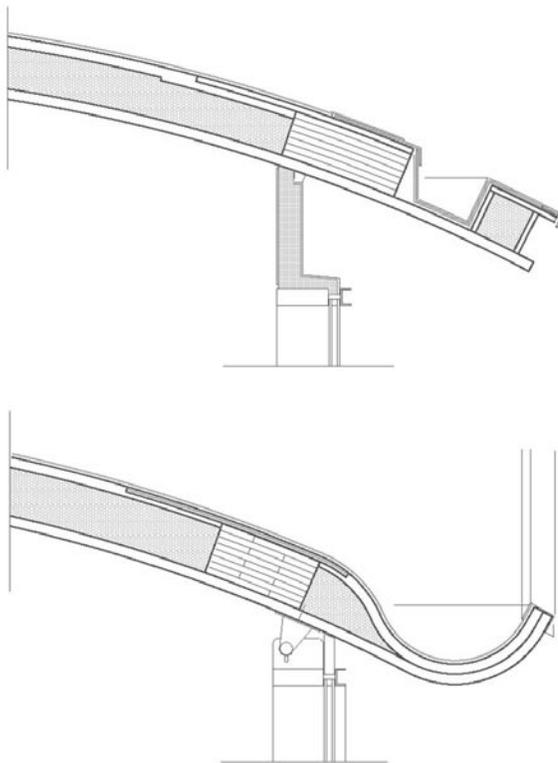
Figure 8. Possible edge details of a Wood-Foam Sandwich shell
