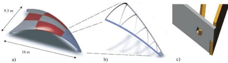
Figure 9. The shell is subdivided into segments (a). A triangulated network of steel ribs is parametrically modeled (b). The slotted connection, modeled with a custom macro (c).
