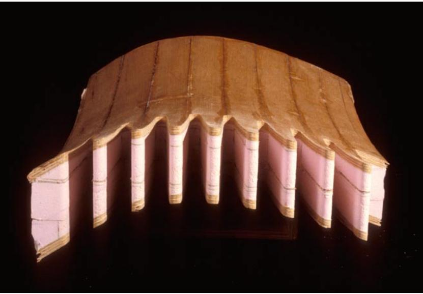
Figure 7. Prototypical sandwich shell panel with a milled fingerjoint
