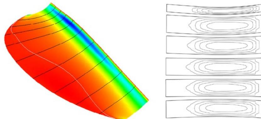
Figure 5. Left: The width and depth of wood strips are derived by determining the internal strains based on the curvature analysis. Right: Digitally flattened strips
