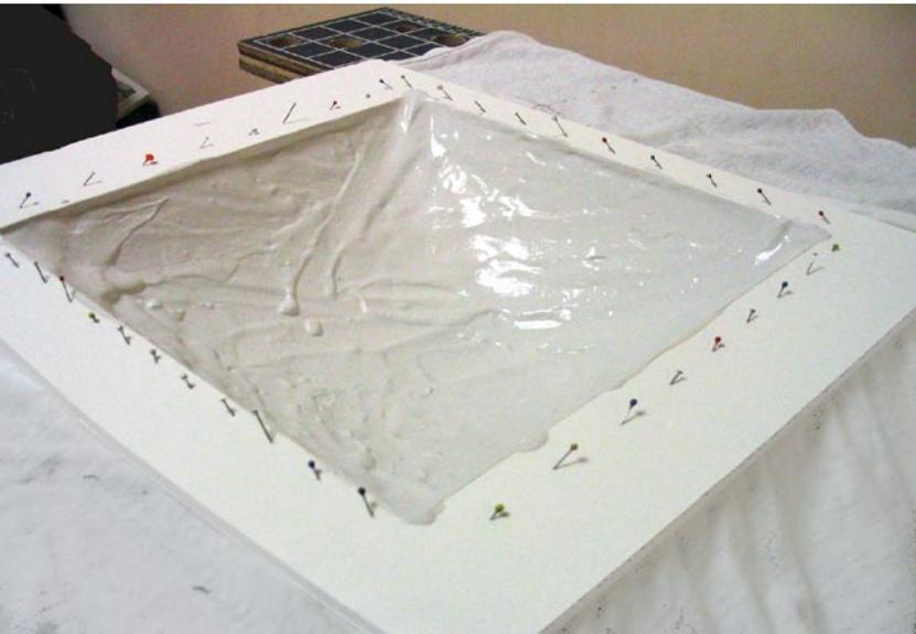
Figure 1. Conceptual physical formfinding model: a hanging fabric, supported continuously along its edges, is coated with plaster. As the fabric has to carry the weight of the material, it automatically takes on a funicular equilibrium shape. Each change in loads or support conditions would yield a different shape.
