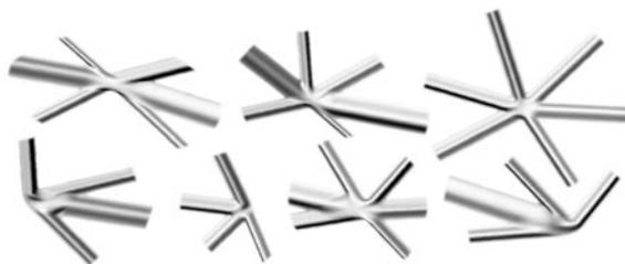
Figure 6. Joint studies from a previous project for intersections of members of unequal diameter in different spatial configurations using a parametric representation
