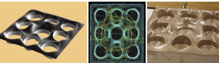
Figure 18. Digital model, tool path geometry, and mold for bubble wall. Sharad Sharma, Beth Jagnow, Emily Fischer
