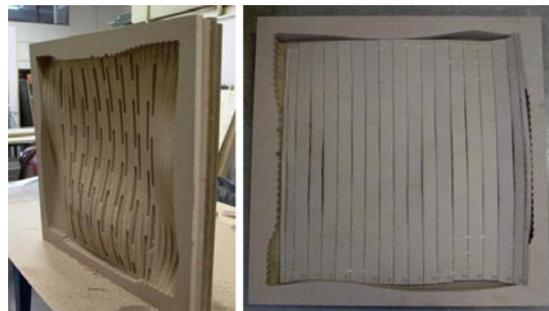
Figure 9. Milled surface model and flattened laser cut paper surface
