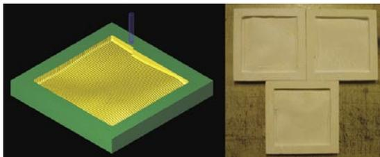
Figure 4. Simulated tool path used for 3D printing.
