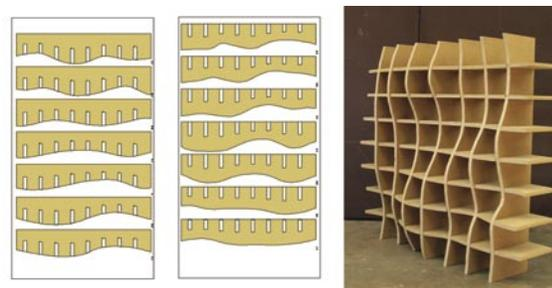
Figure 6. Cut Sheet and CSP Construction.
