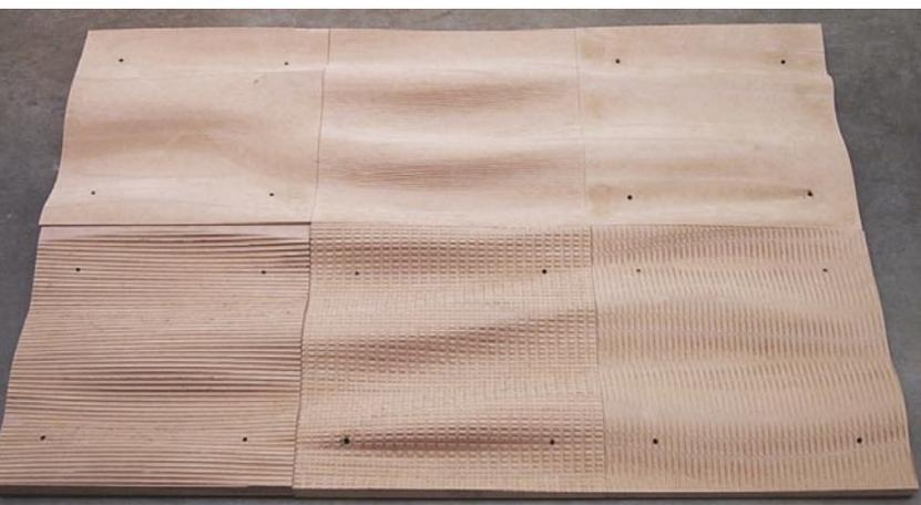
Figure 12. Each team was required to mill a surface that would fit next to another team's. Image shows all six surfaces arranged in order, each team using a different finish toolpath.
