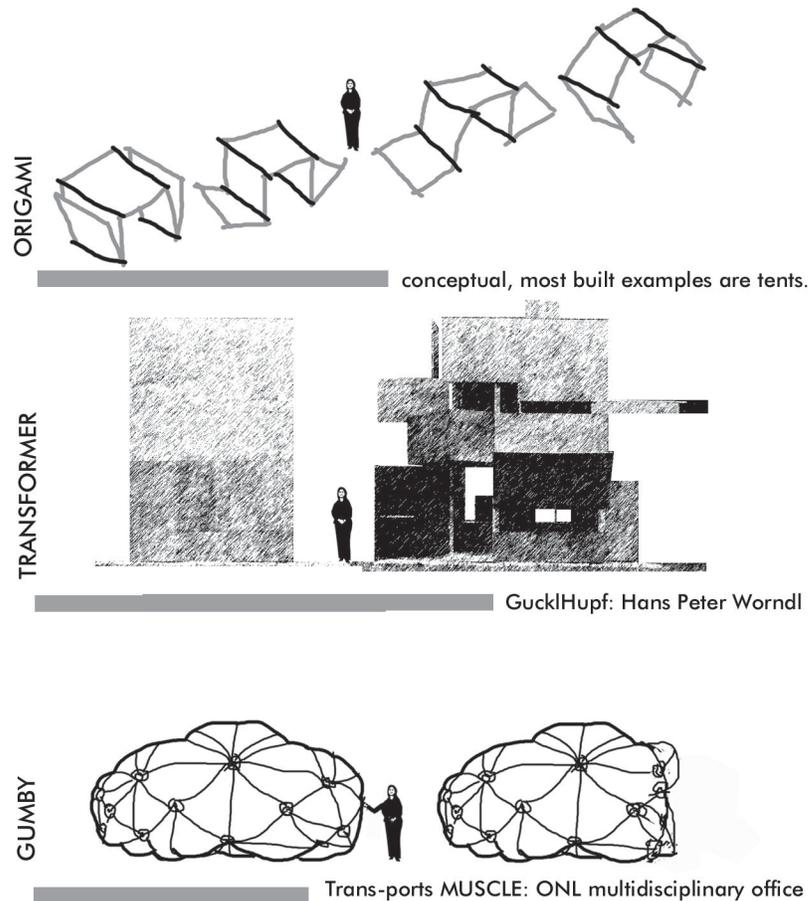
Figure 3. The three types of transformation of an adaptive kinetic structure
