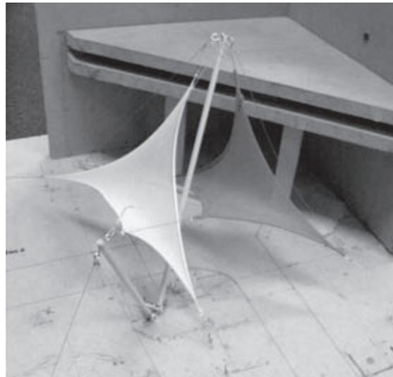
Figure 8. Physical Stretch Model for Exploration.
