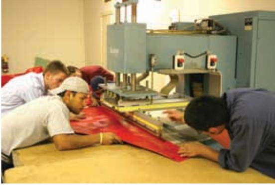
Figure 7: Radio Frequency Welding of Fabric Panels.
