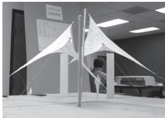
Figure 9. Physical Patterned and Welded Model for Verification.
