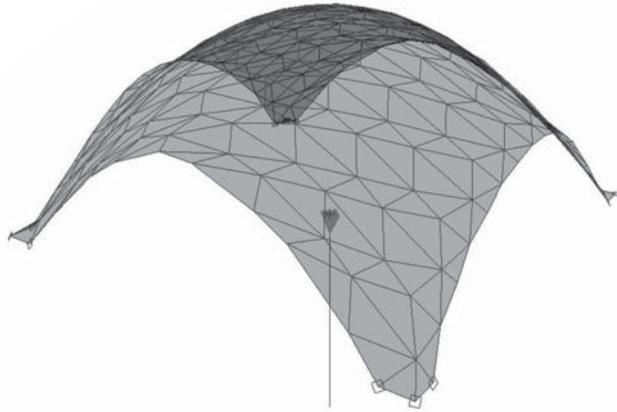
**FIGURE 3** Catenary network drape form using dynamic cloth simulation
