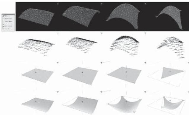
**FIGURE 5** CS-FEM form analysis showing constrained edges and points
