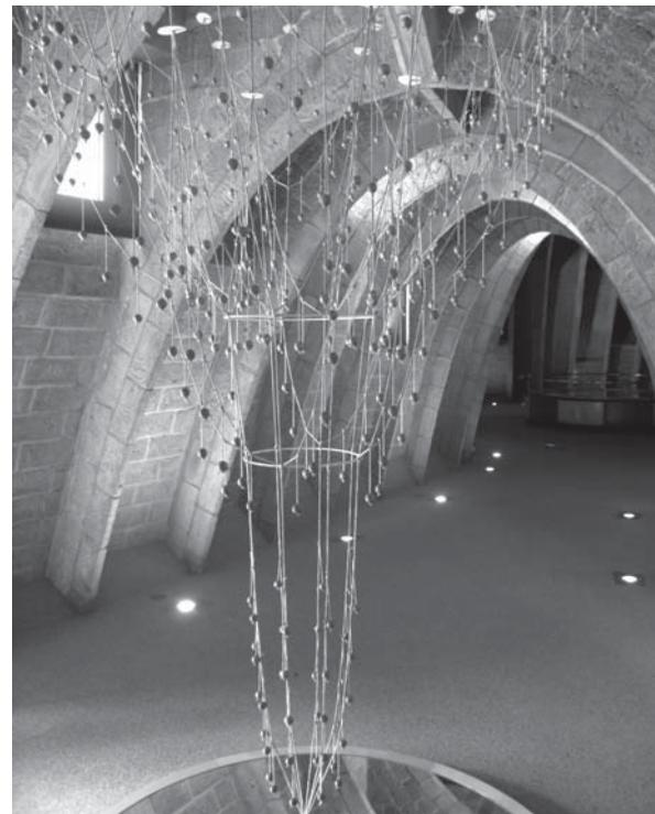
**FIGURE 2** Catenary string model showing method for form finding of optimal force path network per given loading condition
