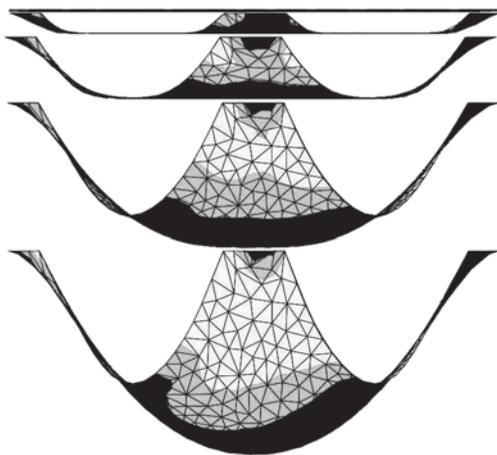
**FIGURE 4** Cloth catenary model composite showing stages of draping simulation
