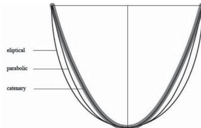
**FIGURE 1** Catenary curve diagram showing relative difference between elliptical, parabolic, and catenary curves
