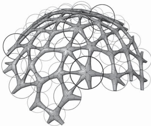
FIGURE 9 Catenary structural network showing locations of ceramic links
