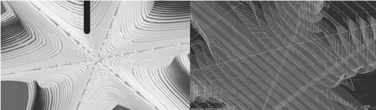
**FIGURE 11** Surface tool paths and cut animation in MasterCAM
