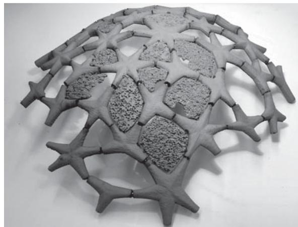
**FIGURE 14** (right) Slip cast scale model of catenary network
