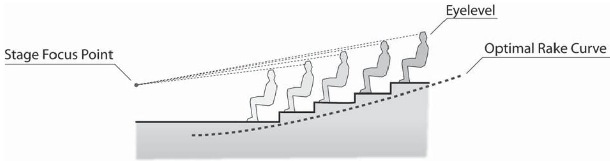
FIGURE 4 The diagram of sight lines.
