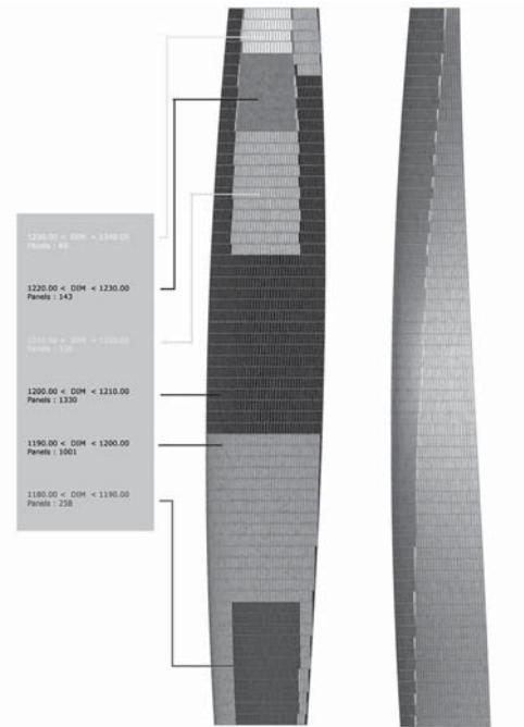
FIGURE 9 Panels grouped and color coded with a 10 mm tolerance in size.
