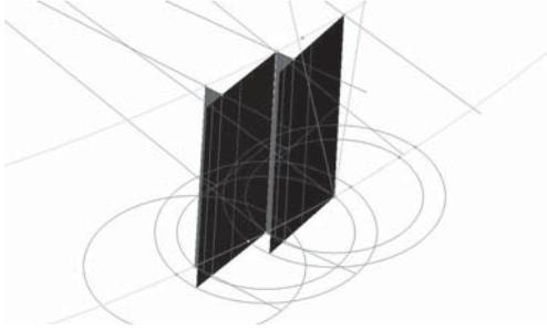
**FIGURE 11** Two consecutive panels and the reference geometries used to locate them in the Cartesian coordinate system. Smaller panels fill the shingle gaps.
