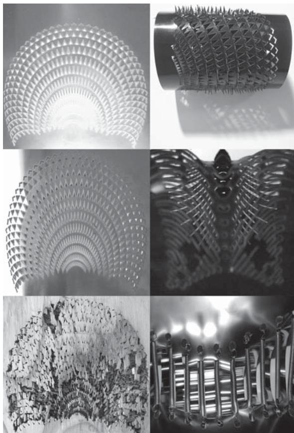
**FIGURE 5** Parallel and nested etching patterns in flexure structures (stainless steel and cut shim stock using the WJC)
