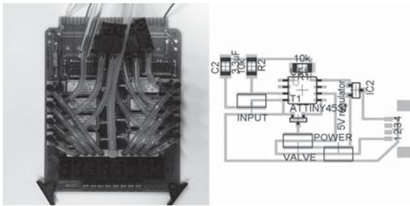
**FIGURE 8** LIGHT-AIR Conversion Protocol: Image shows the solenoid valve board and the circuit board schematics.
