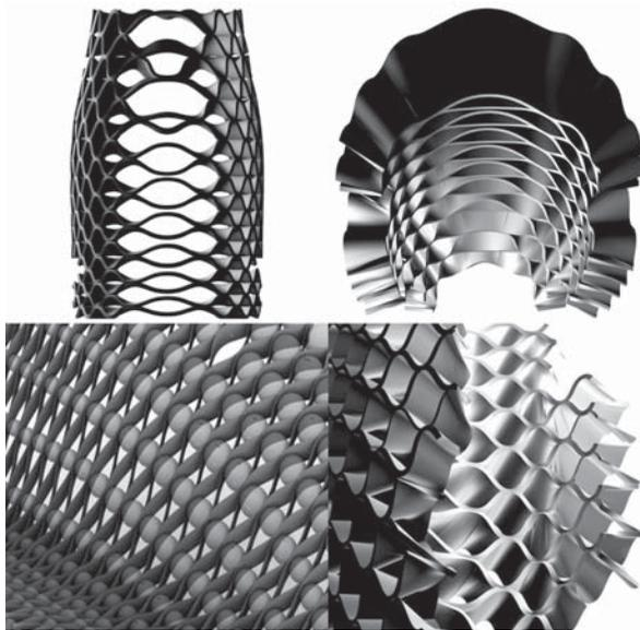
**FIGURE 3** Digital Modeling of Surface Behavior: The model was generated using a parametric software package, where small sphere-like elements increase and decrease volume parametrically to allow for the simulated “stretch” effect of the surface.
