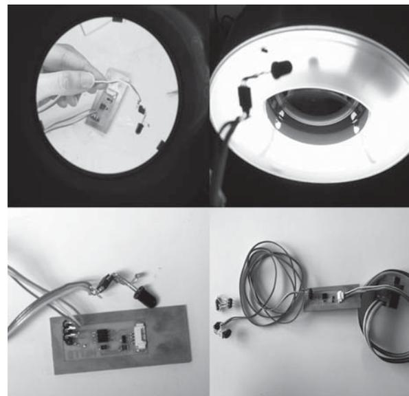
**FIGURE 7** Circuit board and light sensor integration: The circuit was designed to read light levels and convert them into voltage, which in turn would allow for the inflation of bladders within the structure.
