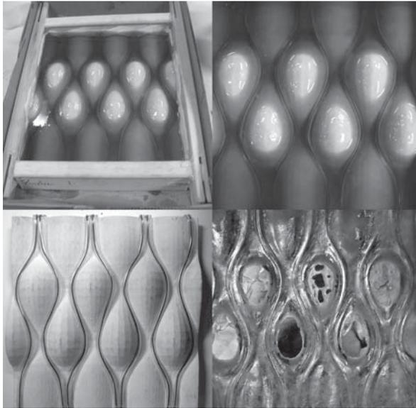
**FIGURE 6** 3-D printed mold with wires (inserted in plastic tubing) The composite structure allows for the incorporation of the structural elements (bent wires) within the skin (rubber), which was designed to allow for inflation "pocket" members.
