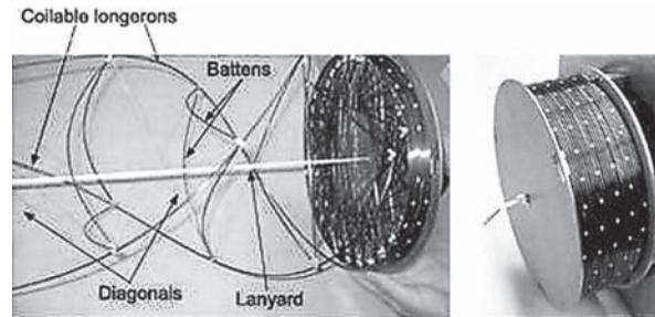
FIGURE 2 NASA coilable mast
