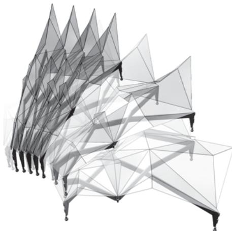
FIGURE 8 A folding structural frame with a rigidly foldable enclosing shell
