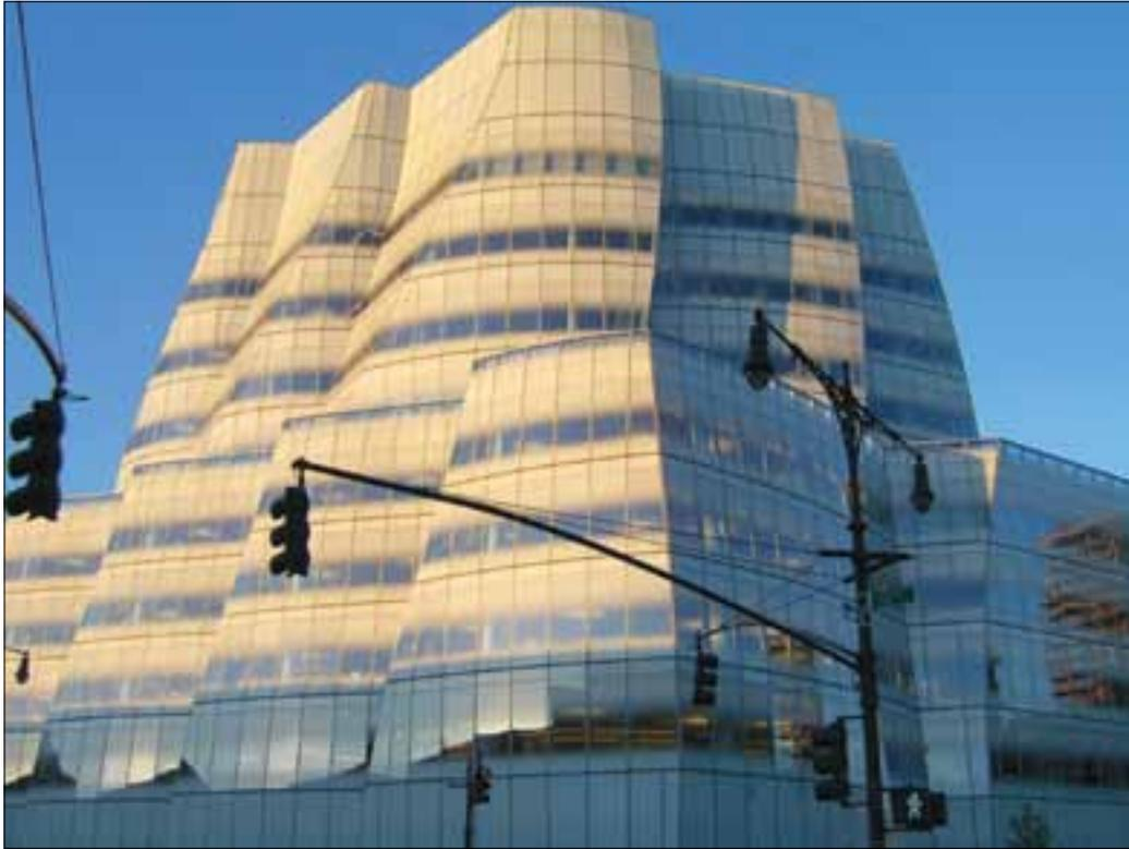
Fritting will block solar gain while letting in diffuse light. Automated versus user-based controls are vital considerations in designing active systems. The design must be robust enough to allow both modes.
