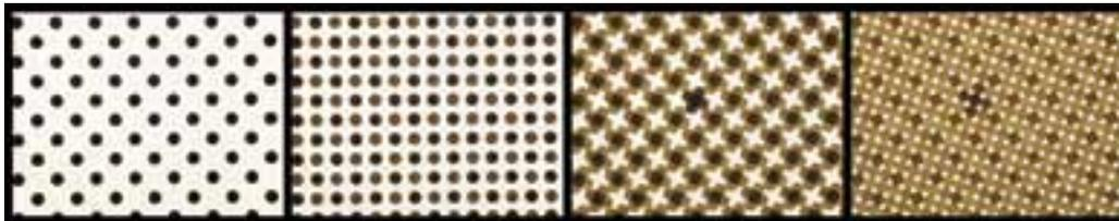
Figure 1 Adjustment of Fritting Density by In-Plane Translation of Stacked Panels.
