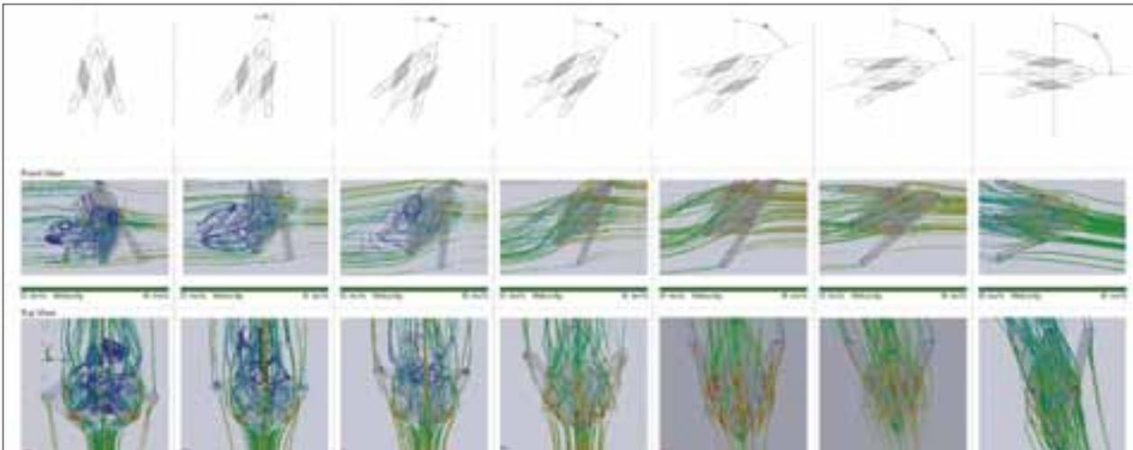
Figure 7 CFD Analysis of the component in different angle variation and opening angle to examine the performance in different circumstances.
