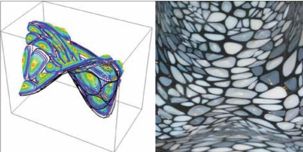
Figure 6 Weighted material selection: a stochastic computational process assigns a stiffness ratio corresponding to environmental performance. The relative height of the soft silicon bumps corresponds to the body pressure mappings.
