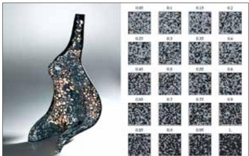
Figure 5 Weighted material selection: a stochastic computational process assigns a stiffness ratio corresponding to structural performance
